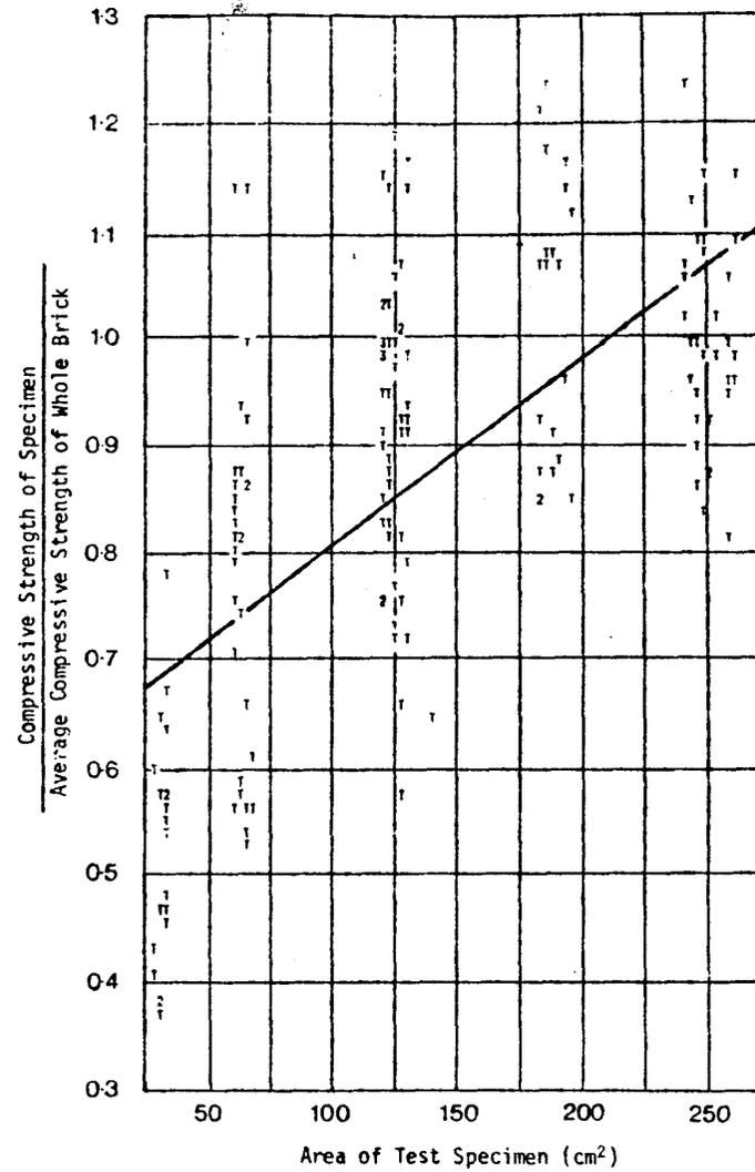
Figure 4.1.3. Plot of observed compressive strengths: Extruded bricks type 1
