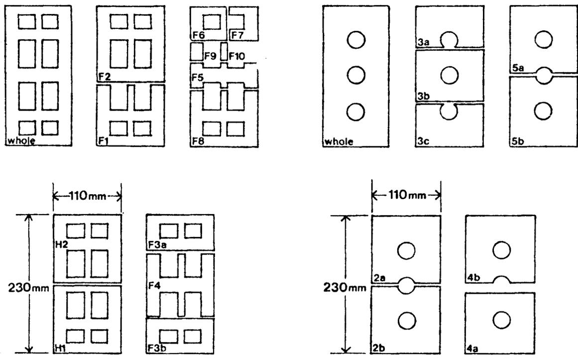
**Figure 3.1.1 & 3.1.2. Wholes and fractions extruded bricks type 1 (left) and type 2 (right)**
