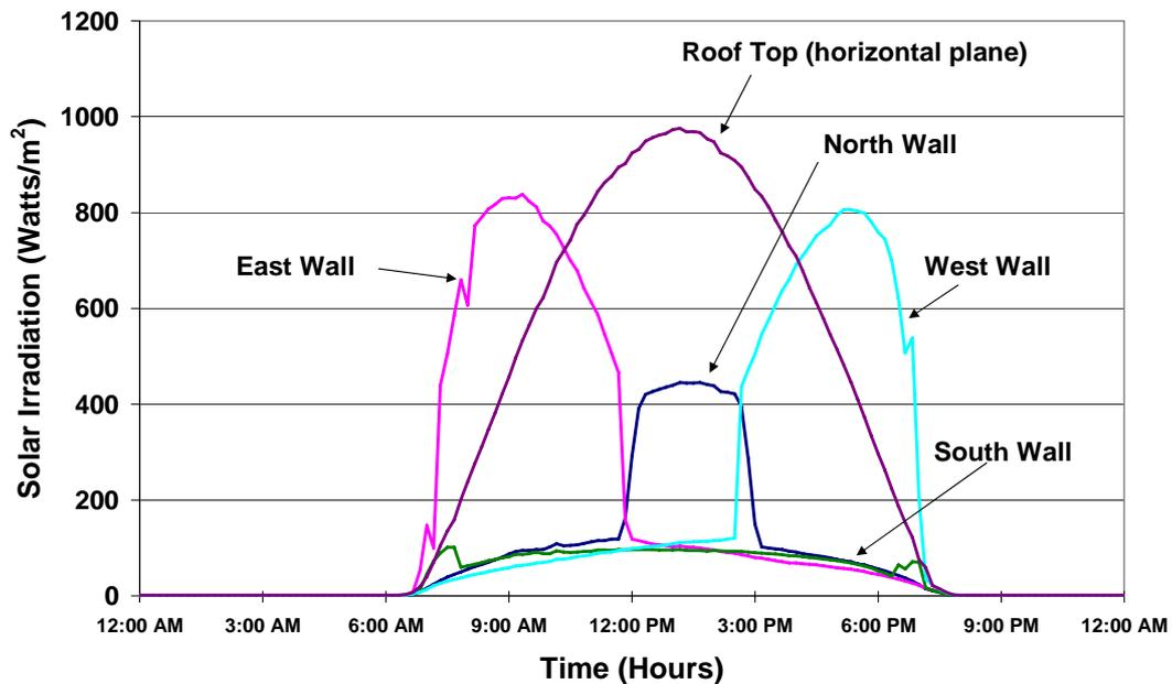
Figure 7. Incident solar irradiation on the exterior building surfaces, 20<sup>th</sup> February 2004.
