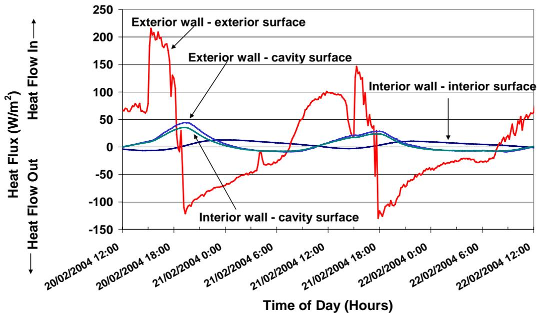
Figure 9. Through-Wall Heat Flux Profile of the West walls of the Cavity Brick Building on the 21<sup>st</sup> February 2004.
