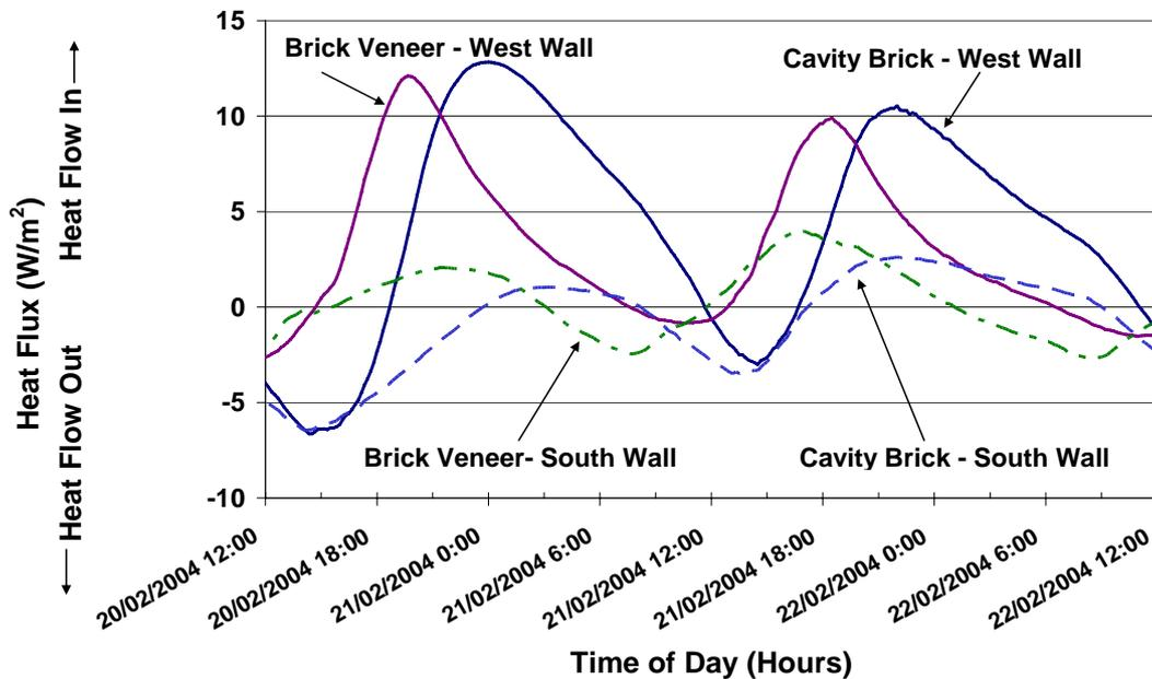
Figure 8. Heat Flux Measurements on the Interior West and South walls of the Cavity and Brick Veneer Buildings for 21<sup>st</sup> February 2004.
