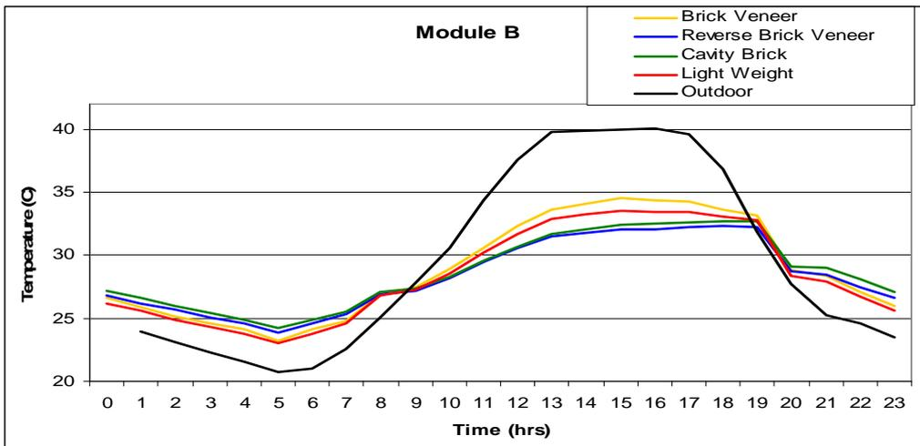
Figure 2: Temperature Profile for Module B in Summer
