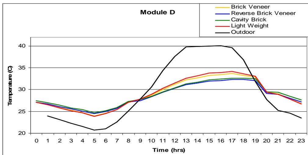
Figure 4: Temperature Profile for Module D in Summer
