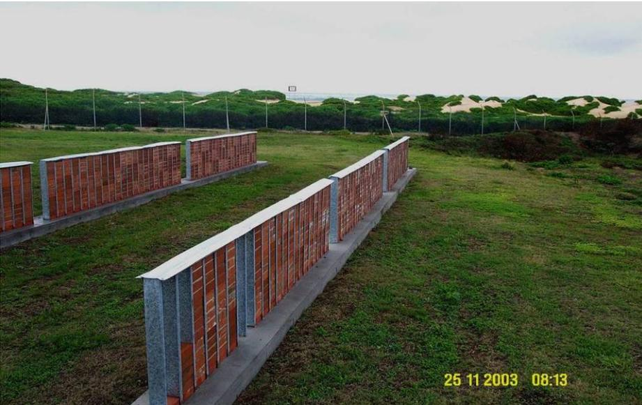
Figure 2. Test Specimens in the Exposed Environment
