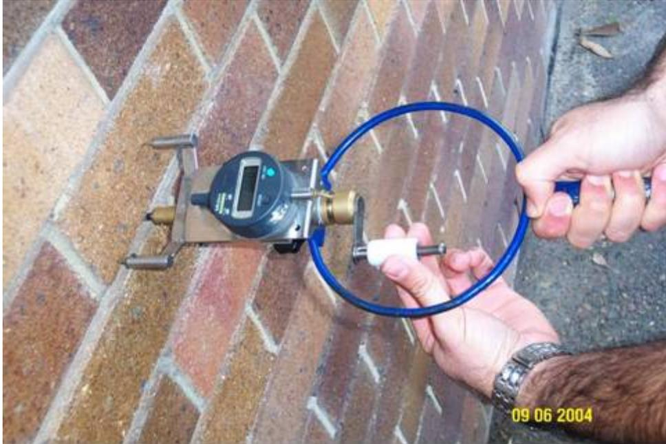
Figure 3. A Scratch Test Performed on a Wall
