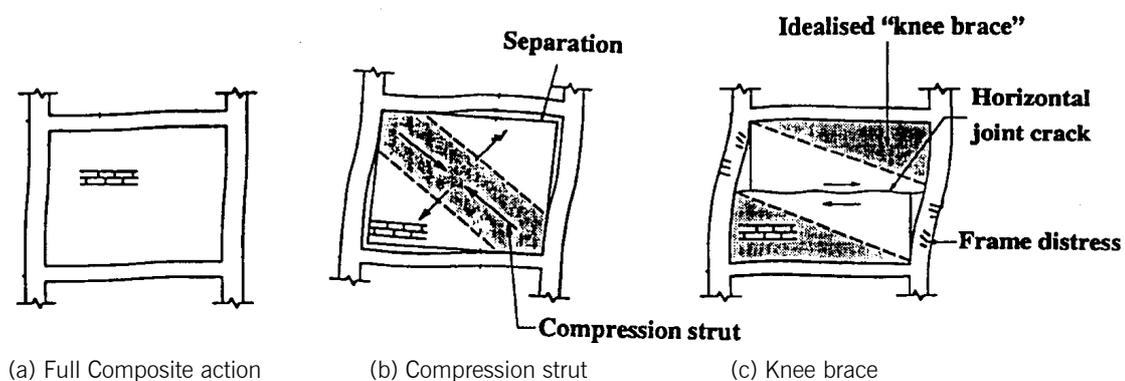
**Figure 7. Behaviour of masonry infill (after Dysdale *et al*<sup>3</sup>)**
