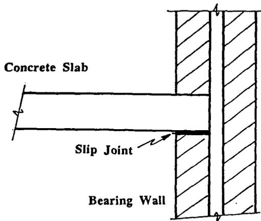
Figure 5. Typical Slab-Wall Connection
