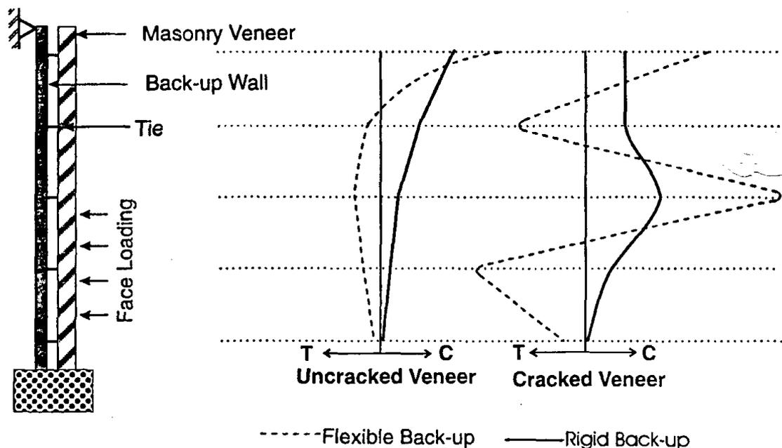
Figure 6. Variation in tie forces for masonry veneers
