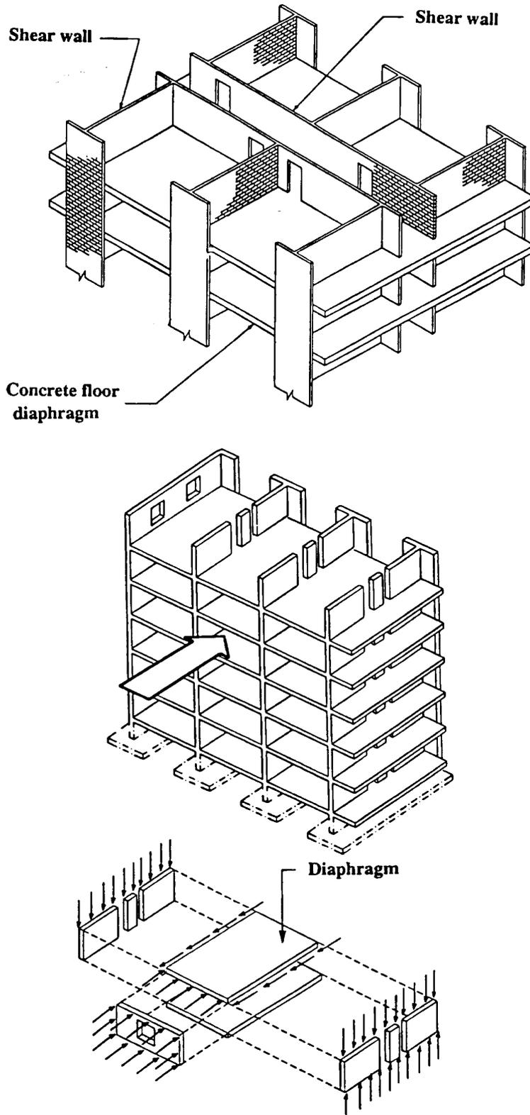
The seismic performance of a loadbearing structure will predominantly depend upon its lateral load resistance. The basic mechanism of lateral load transmission for a loadbearing structure is shown in Figure 1. The lateral load will either be applied to the structure by wind or induced in the structure by earthquake ground movements.
