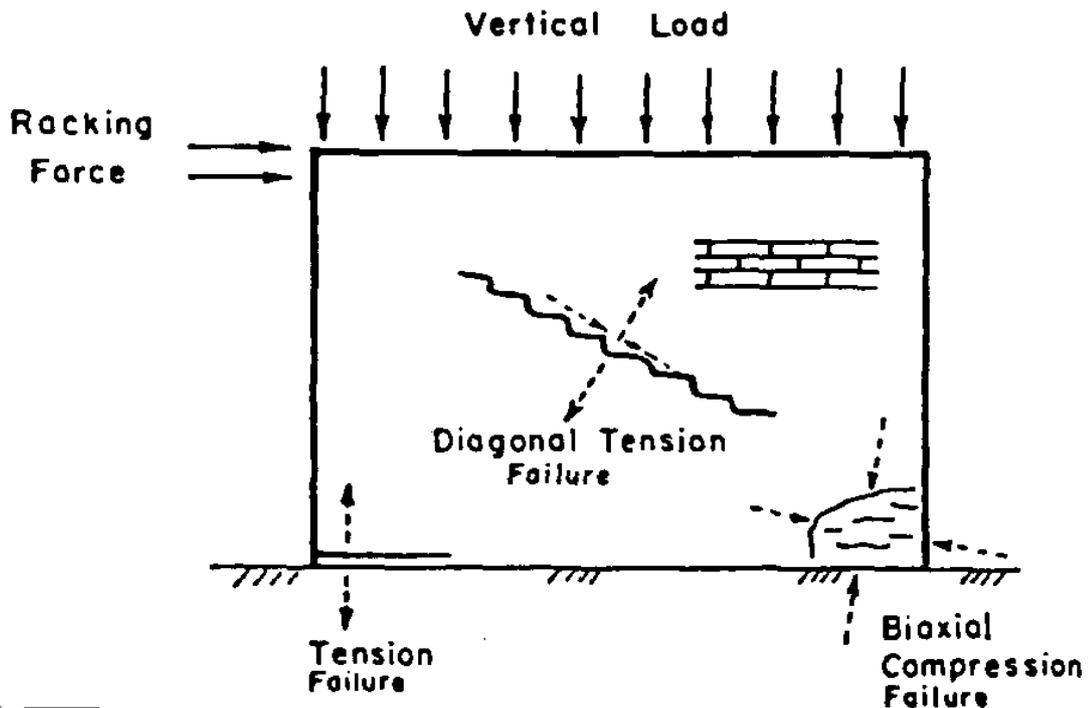
**Figure 4. Modes of Failure for a Shear Wall**
