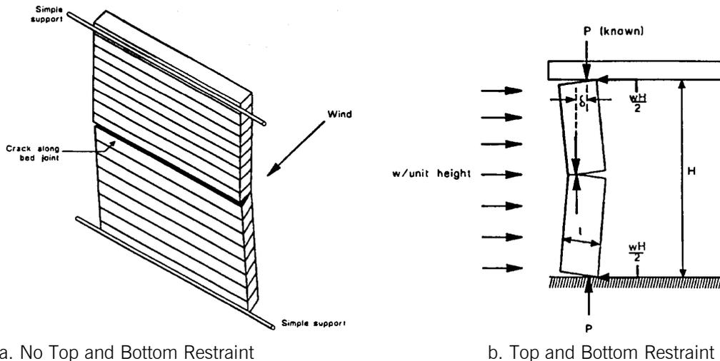
**Figure 2. Lateral Load Behaviour of Vertically Spanning Walls**
