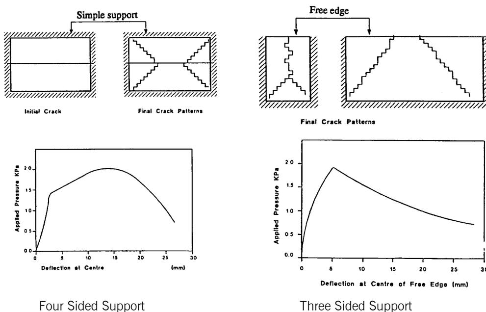
**Figure 3. Lateral Load Behaviour of Two Way Spanning Walls**
