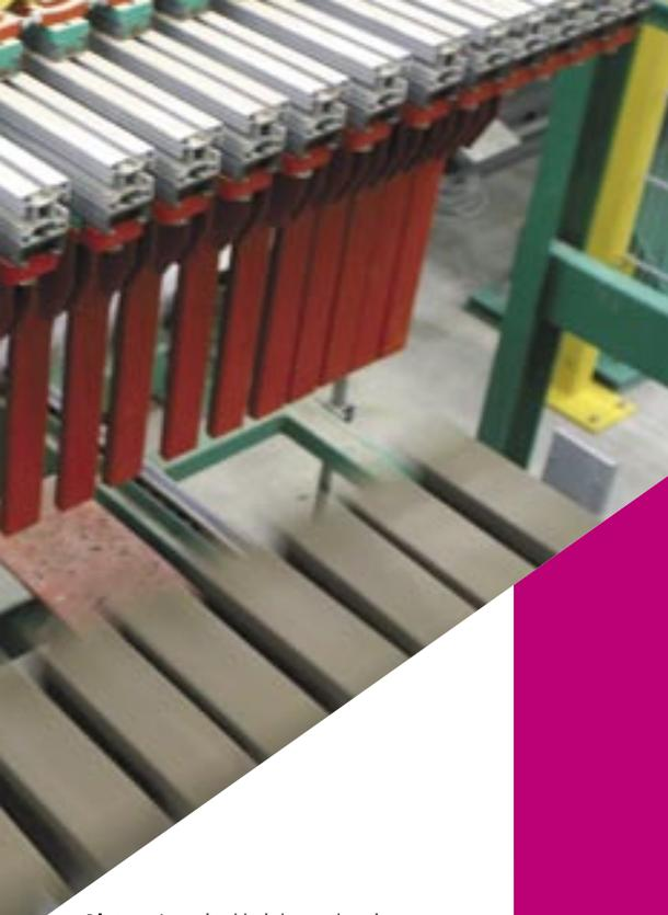
**Above** A typical brick production line showing the 'green' (unfired) units travelling at high speed down a conveyor system.
