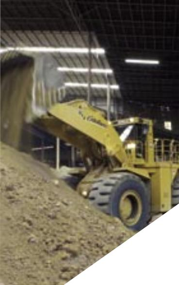
**Above** Heavy earthmoving machines are used to extract and stockpile clay.
